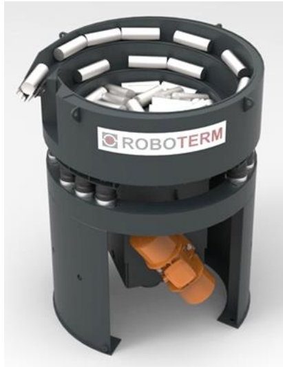
Fig. 1 - Vibratory bowl feeder for automatic feeding of billets into forging lines
