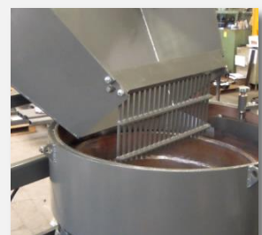
Bin tipper filling
