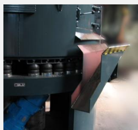
Side emptying chute
